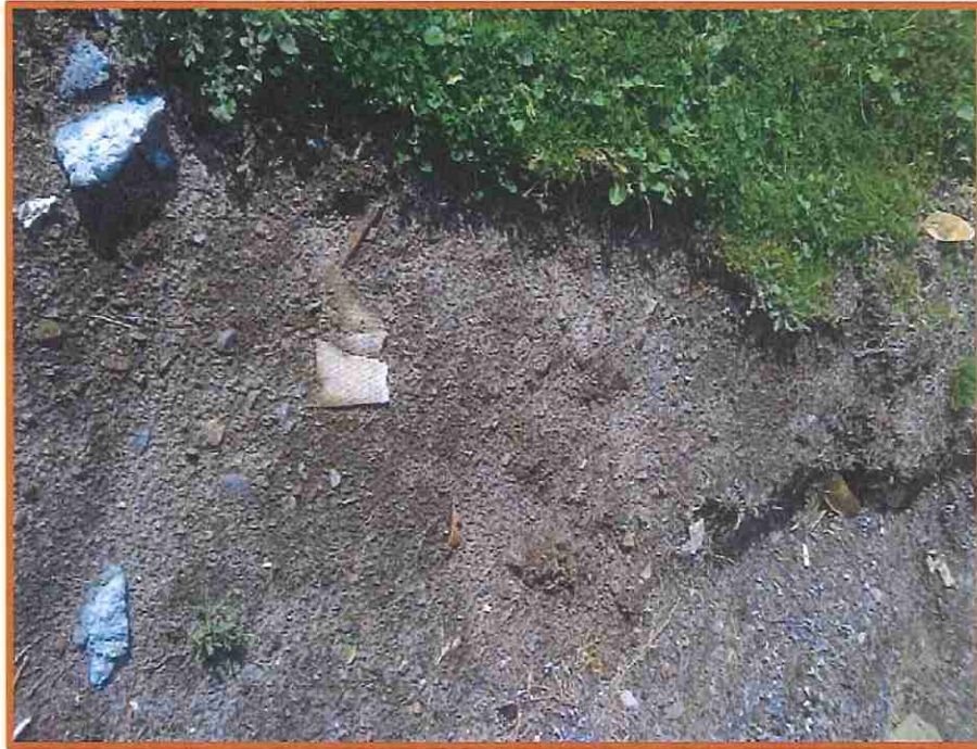
Figure 1 Example of Asbestos Containing Material (ACM)
